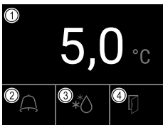
Fig. 63 Status display (1) Actual temperature (2) Alarm status (3) Defrosting status (4) Door opening status
