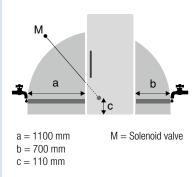
Plumbing must be installed adjacent to the side of the appliance which contains the lceMaker. Water pressure must be between 0.15 MPa and 0.6 MPa (1.5 bar - 6 bar)
