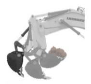
**Semi-automatic bucket filling function** Allows the machine electronic to realise fully automatic attachment movements.
