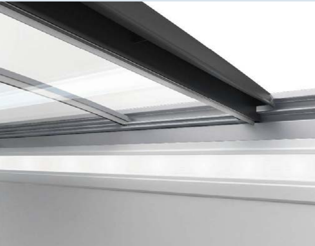
Smooth-running sliding glass lid. The curved sliding glass lids on the EFI chests are made of toughened, single-pane safety glass. The lid halves are easy to move thanks to profiled seals and the plastic frame heated by hot gas from the compressor.
