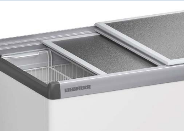
Insulated sliding lid. The sliding foam lids range are extremely robust thanks to the composite aluminium and rigid PVC cover. The top is protected with a scratch-resistant aluminium worktop. Insulated sliding foam lid is available as an alternate option to the flat sliding glass lids. A lid lock is available as an accessory.
