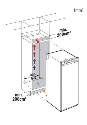
Figures 1, 2 and 3 represent the alternate ways that Liebherr single door or double door integrated appliances can be installed to ensure correct ventilation requirements are achieved.
