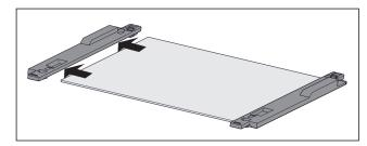
Fig. 127 Glass shelf with retaining part
