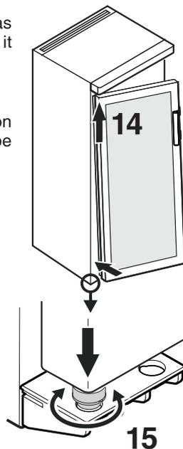
18. Undo screws and slide hinge bracket to the right or left. Tighten screws.
