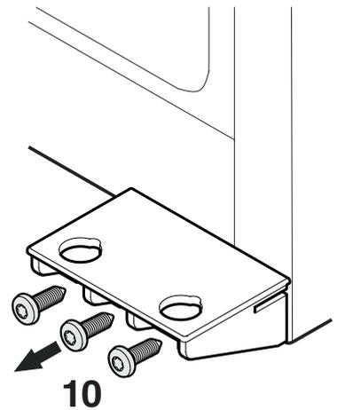
11. Remove the cover, turn it through 180° and re-fit it on the opposite side.
