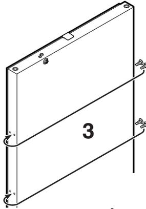
4. Transfer pin on hinge bracket to the opposite side.
