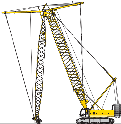
Erecting of main boom and luffing jib
