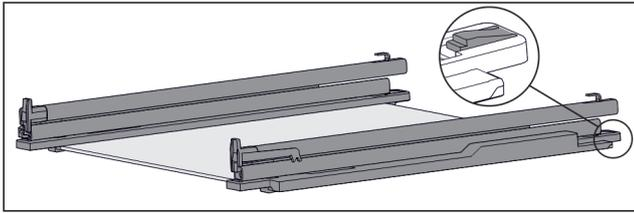
Fig. 43 Glass shelf with rails and retaining parts
