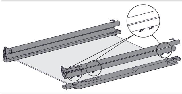
Fig. 44 Glass shelf with rails and retaining parts
