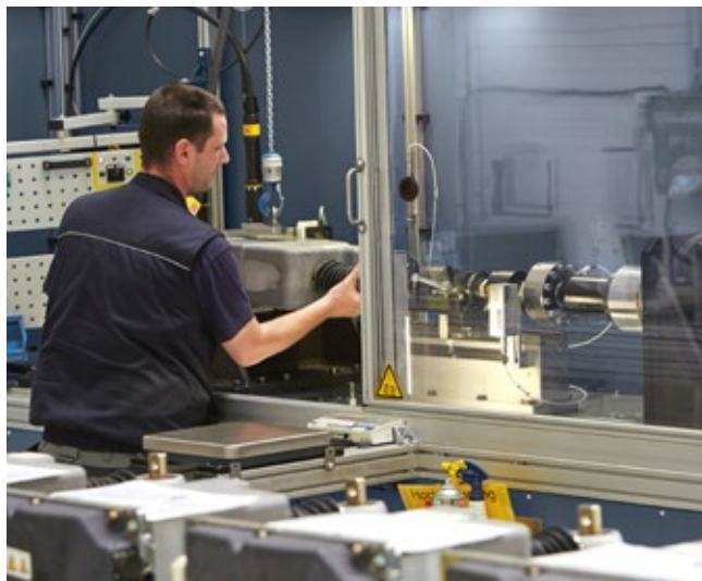
An electro-hydraulic actuator is prepared for testing.
