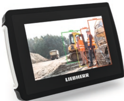
Distance to the obstacle is outlined on the monitor screen
