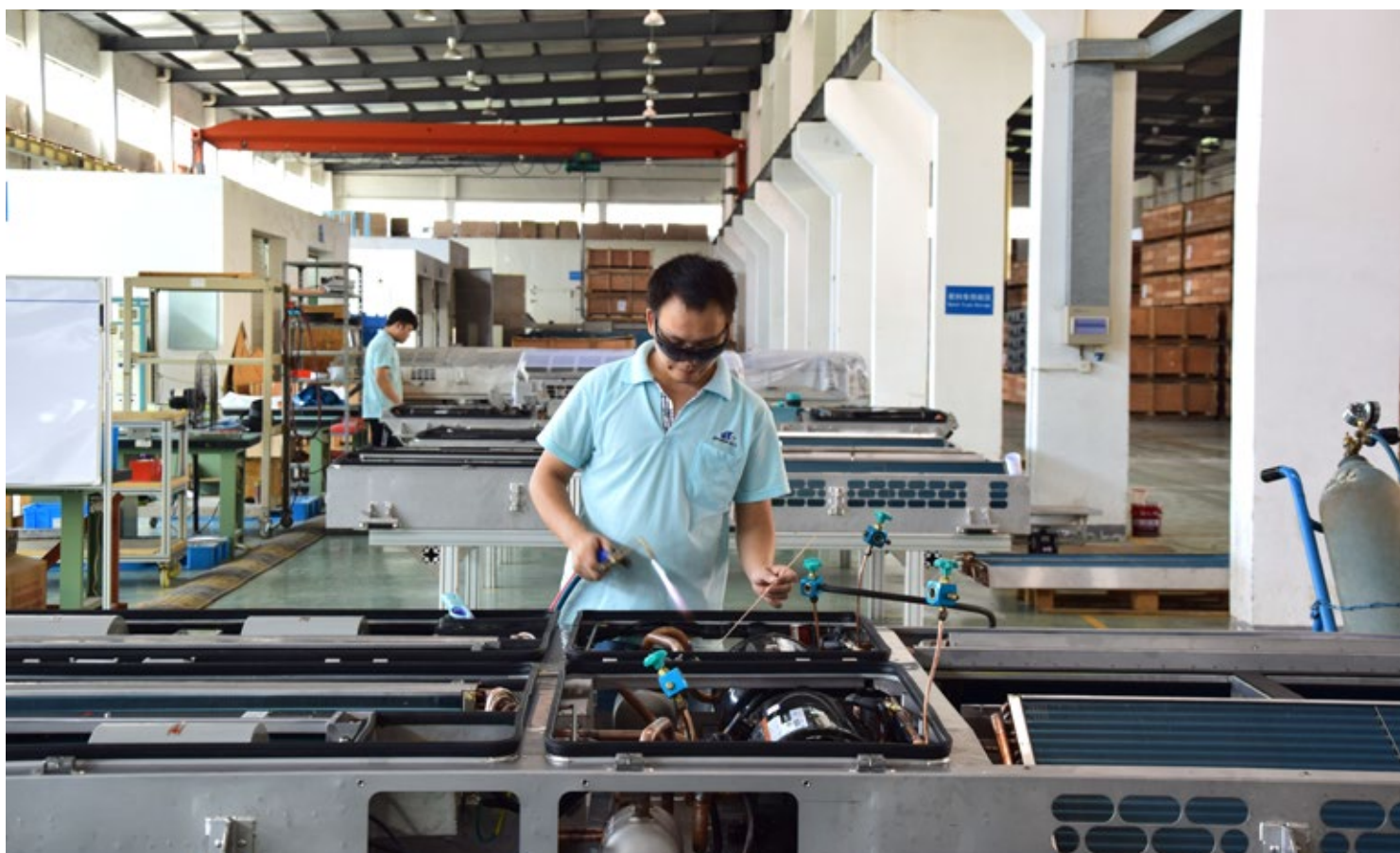
Production islands instead of conveyor belts: in this way, the company can react quickly to new requirements or small series requests.
