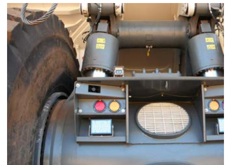
Service door on axle box for inspections
