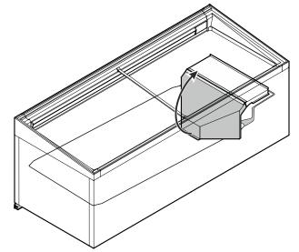
• Pull up the fan cover and clean the defrost drain gulley beneath it.
