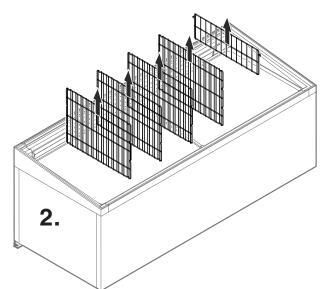
Removing the separators if there is a shortage of space due to display units above the appliance • Unhook one of the support brackets,
