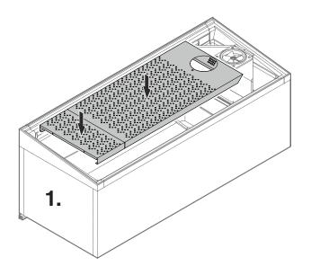
Close the fan cover. Slide the baseplate until the rectangular openings are precisely over each other. Push the pin into the opening from the top.
