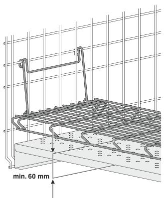
Important note The storage grids must be fitted. No goods may be placed on the baseplates.
