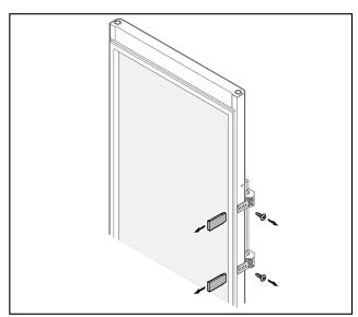
Fig. 36 Glass door\* Remove the panels. Unscrew the handle.
