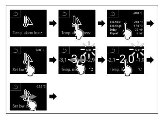
Fig. 185 Example of setting the lower temperature limit based on a set appliance temperature of -20 °C.
