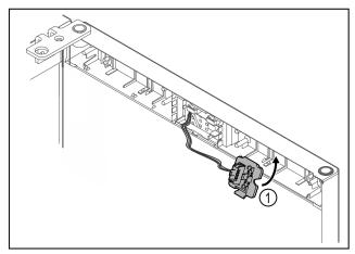
▶ Snap in the plug holder Fig. 23 (1) on the opposite side.
