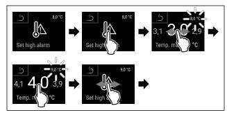
Fig. 179 Example of setting the lower temperature limit based on a set appliance temperature of 5 °C.
