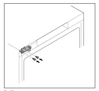
Fig. 29 ► Move the hinge to the opposite side.
