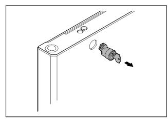
Fig. 44 ▶ Pull out the lock.
