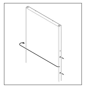
Fig. 37 ▶ Put the stopper on the opposite side.
