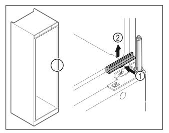
▶ Gently press the middle of the cover Fig. 31 (1) and lift it off Fig. 31 (2).
