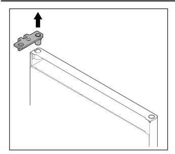
Fig. 26 ▶ Pull out the hinge.
