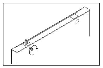
Fig. 42 Freezer compartment door ► Engage the lock.
