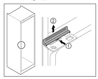
Gently press the middle of the cover Fig. 48 (1) and lift it off Fig. 48 (2).
