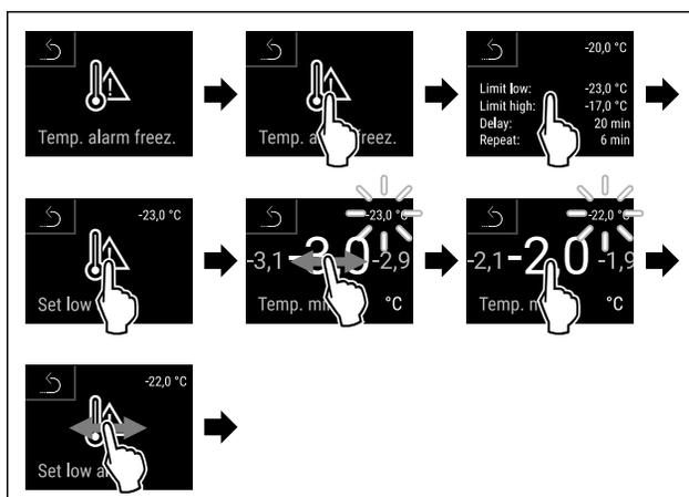
Fig. 169 Example for setting the lower temperature limit based on a set appliance temperature of -20 °C.
