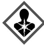
The symbol may be located on the compressor. It refers to the oil in the compressor and refers to the following danger: **Can be fatal if swallowed or inhaled.** This notice only applies for recycling. There is no danger during normal operation.
