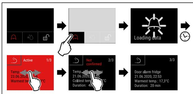
Fig. 225 Example shows an active alarm, an unconfirmed alarm, and a confirmed alarm.
