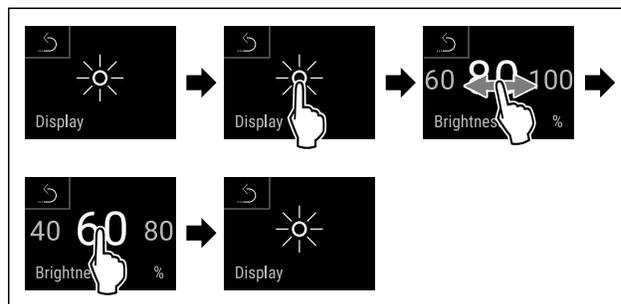
Fig. 121 Example illustration: Switching from 80% to 60%.
