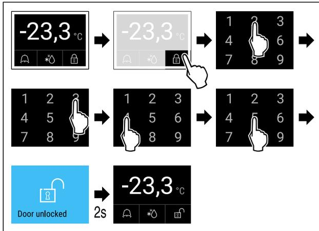
Fig. 223 Example shows PIN 2345
