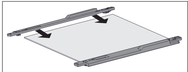
*Fig. 67 Glass shelf with retaining part*
