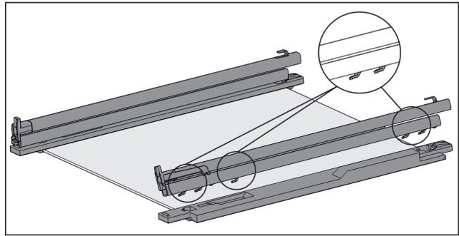
*Fig. 65 Glass shelf with rails and retaining parts*
