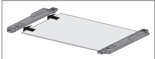
*Fig. 66 Glass shelf with retaining part*
