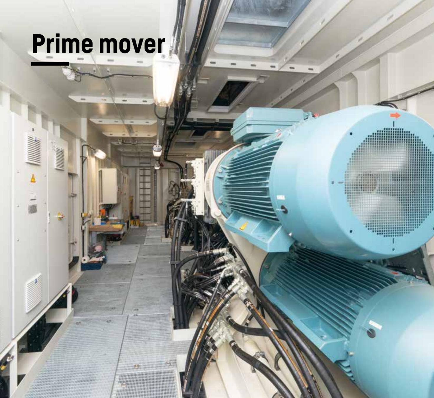
The crane design offers the customer a choice of diesel-hydraulic or electric-hydraulic drive to best meet project requirements.
