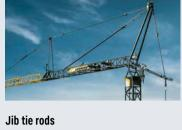
Guying the jib using tie rods ensures safe erection and high stability in operation.
