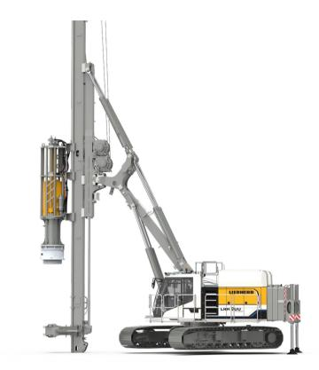
By supporting the leader on the ground and extending the rear support cylinders, the carrier machine is elevated. The undercarriage can thus be swivelled on the spot, which makes it easier to move the piling rig in restricted spaces.
