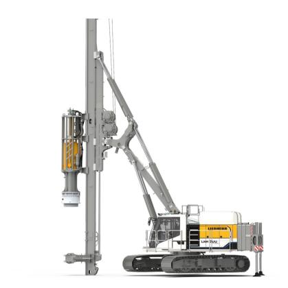
By supporting the leader on the ground and extending the rear support cylinders, the carrier machine is elevated. The undercarriage can thus be swivelled on the spot, which makes it easier to move the piling rig in restricted spaces.
