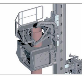
Ring vibrator with platform and concreting system
