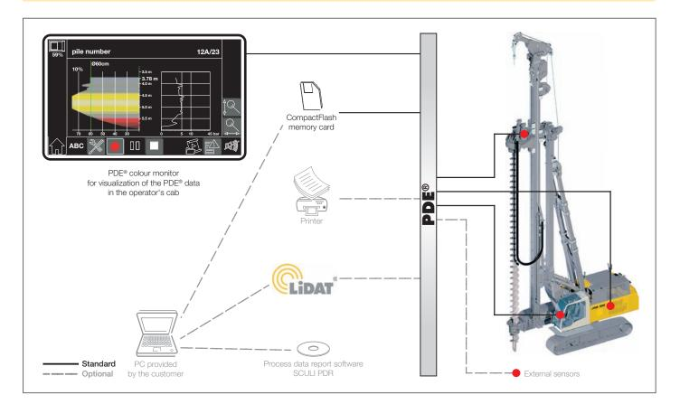
Depending on the application the recorded and processed data are displayed on the PDE® touchscreen in the operator's cab, e.g. in the form of an online cast-in-place pile.
