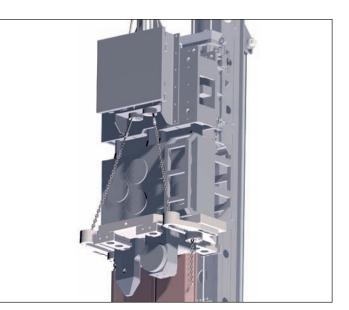
Double clamp and hydraulic sheet pile feeder
