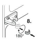
**8.** Remove hinge bushing, turn through 180° and re-fit.
