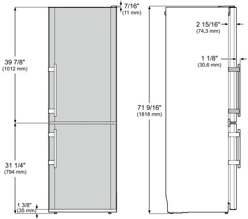
Overall height of the appliance can be increased by a maximum of 5/8" (see Leveling the appliance).
