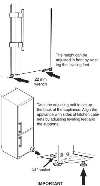
After final installation, this screw must be turned down until it has proper floor contact to support the hinge bracket.
