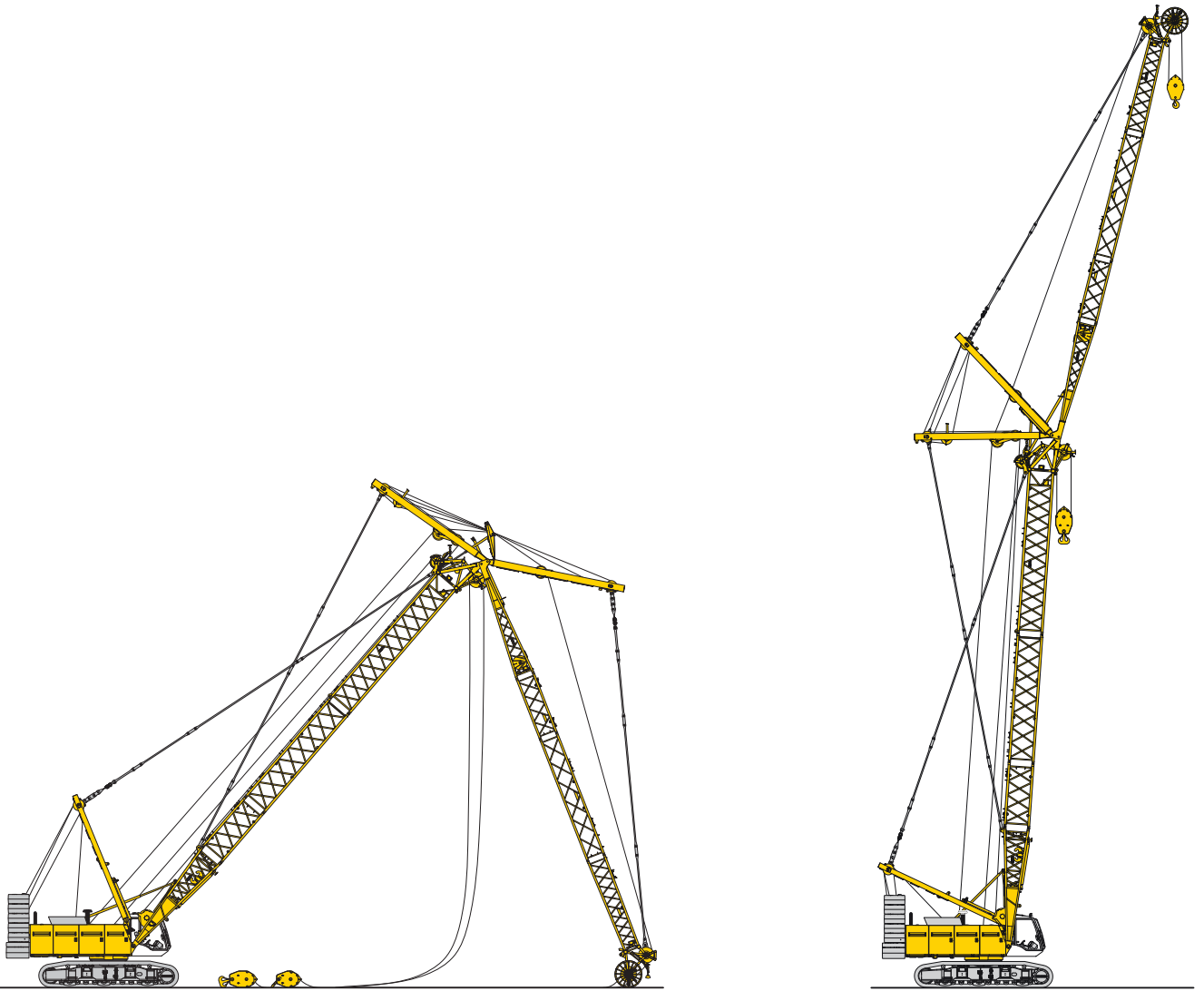
Erecting of main boom and luffing jib
