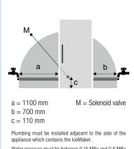
Water pressure must be between 0.15 MPa and 0.6 MPa (1.5 bar - 6 bar)
