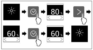
Fig. 48 Example illustration: Switch from 80 % to 60 %.
