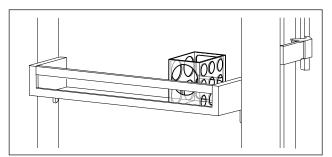
Fig. 120 Example illustration ► Insert the FlexCube in the door rack. -or-
