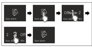
Fig. 57 Example illustration: Changing the door alarm from 1 minute to 3 minutes.
