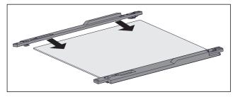
Fig. 123 Glass shelf with retaining part
