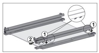
Fig. 125 Glass shelf with rails and retaining parts Install rail with damping mechanism:
