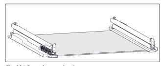
Fig. 124 Damping mechanism
