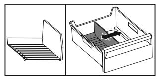
Fig. 108 Example illustration of the ice compartment divider
