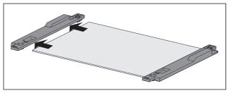
Fig. 122 Glass shelf with retaining part
