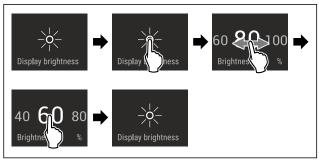
Fig. 55 Example illustration: Switching from 80 % to 60 %.
