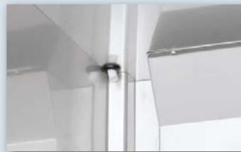
Laboratory appliances with electronic controls and top mounted cooling systems are equipped with an access port (7 mm / 9/32" in diameter) in the top compartment for **connecting independent temperature sensors.**
