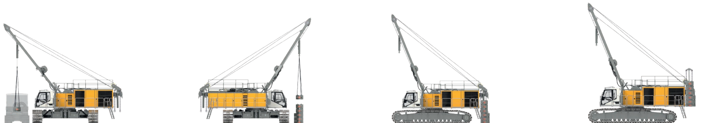
Unloading and assembly of rear counterweight
