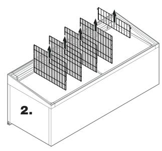
Removing the separators if there is a shortage of space due to display units above the appliance
