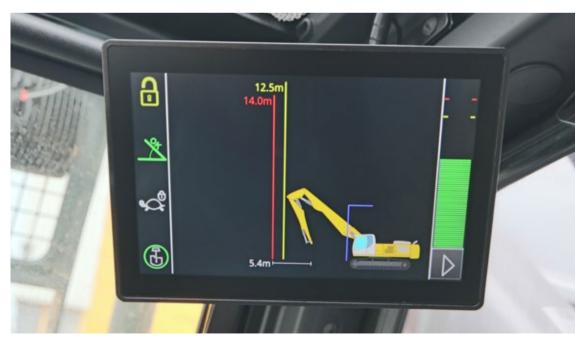
The LDC system is ergonomically arranged in the operators field of view so that it is easy and fatigueless to monitor. If a critical measure value is exceeded the LDC system auto-
