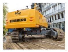
Hydraulically adjustable undercarriage
