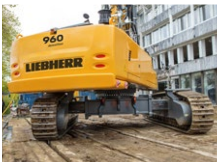
Hydraulically adjustable undercarriage for easy transportation and wider working foot print for stability
