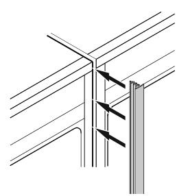
13. Open the doors and press the cover strip into the gap between the appliances.
