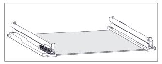
Fig. 120 Damping mechanism
