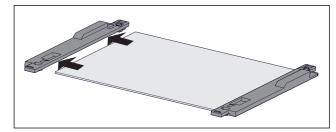
Fig. 118 Glass shelf with retaining part
