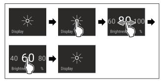
Fig. 60 Example illustration: Switch from 80 % to 60 %.
