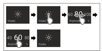
Fig. 50 Example illustration: Switch from 80 % to 60 %. ► Carry out action steps according to the illustration.
