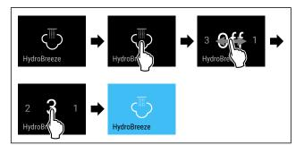
Fig. 43 Example illustration: Activate HydroBreeze with value 3.
