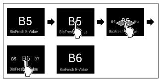
Fig. 26 Example illustration: Switch from B5 to B6.
