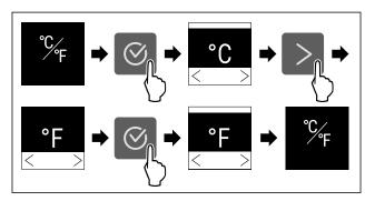
Fig. 23 Example illustration: Switch from degrees Celsius to degrees Fahrenheit.
