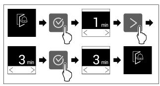
Fig. 58 Example illustration: Change door alarm from 1 minute to 3 minutes.
