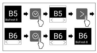
Fig. 25 Example illustration: Switch from B5 to B6.
