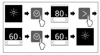
Fig. 56 Example illustration: Switch from 80 % to 60 %.
