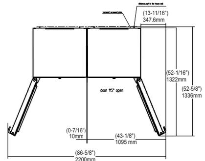
If the appliances are installed with the hinges next to a wall, the distance between the appliance and the wall must be at least 1 1/2" (40 mm). This is how far the handle protrudes when the door is open.
