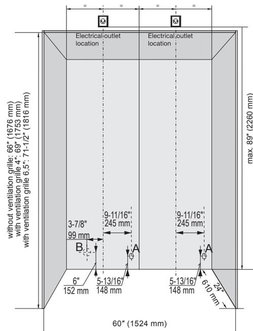
This side by side requires a Side by Side kit to attach both appliances together and provide a finish look.
