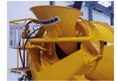
Feeding hopper, mechanically swivelled to the side
