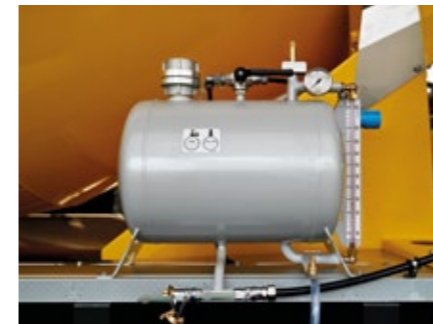
Admixture tank, air pressed
