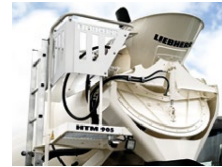
Drum segment lock (3/4 cover), hydraulically operated
