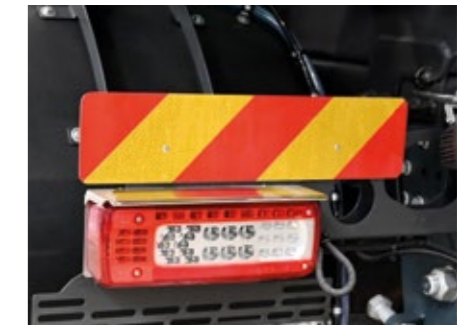
Reflectors above rear lights
