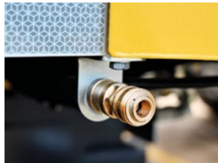
Compressed air connection at the rear
