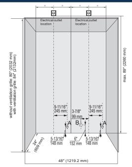
The appliances can be used freestanding or semi built-in. If semi built-in, consider the minimum cabinet opening dimensions specified on this image.
