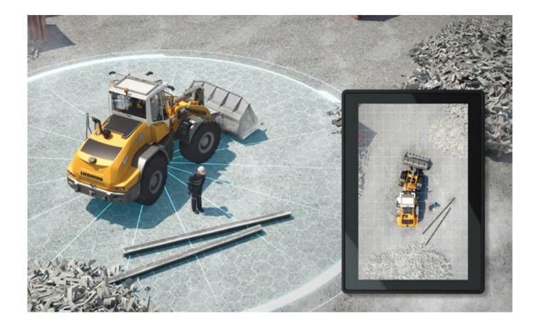
Everything in view – the Skyview 360° system has been fundamentally revised and now has impressive high-definition image quality. The system offers an overview of the whole area around the machine, so that potential hazards can be identified earlier and accidents prevented. The work cycles can be carried out faster, more efficiently and more safely, saving time and money.
