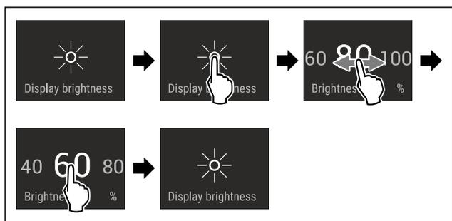
Fig. 48 Example illustration: Switch from 80 % to 60 %.
