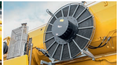
Hose drum for hydraulic cylinder
