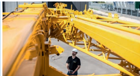
Hydraulic assistance to mount the folding jib with BTT
