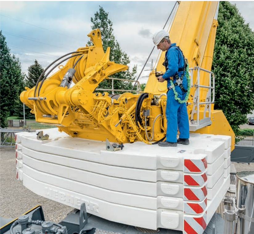
Self-assembly of winch 2 on the LTM 1300-6.2
