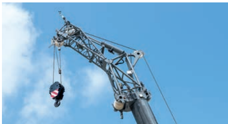
5.5 m integral erection jib, hydraulically adjustable
