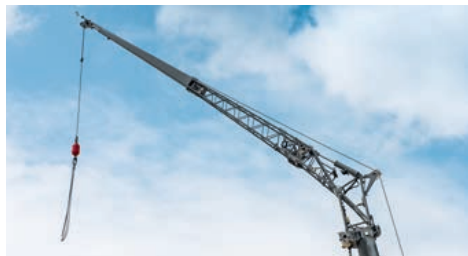
Hydraulically adjustable folding jib (0° to 45°)
