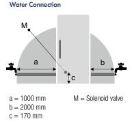
Plumbing must be installed adjacent to the side of the appliance which contains the IceMaker.
