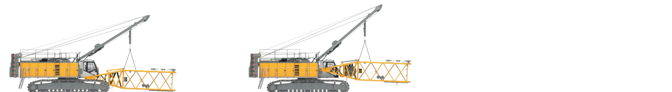
Assembly of boom foot
