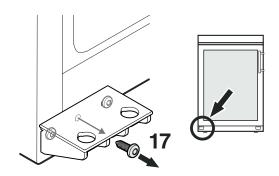
**17.** Remove middle screw from hinge bracket. This screw is no longer needed.
