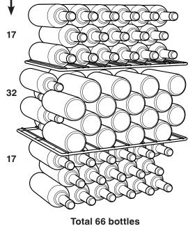
$\angle ! \$  Important The maximum load per grid shelf is 45 kg.
