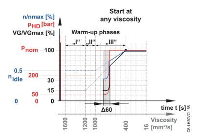
After the 60 s have elapsed, determine the viscosity using the available temperature values and the viscosity chart, select the appropriate warm-up phase and operate the axial piston unit in the defined period and appropriate conditions (see Warm-up phases).
