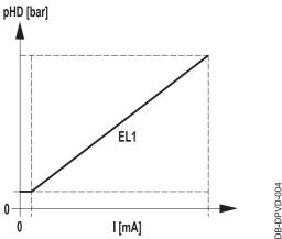
The EL function is designed with a positive characteristic as standard.
