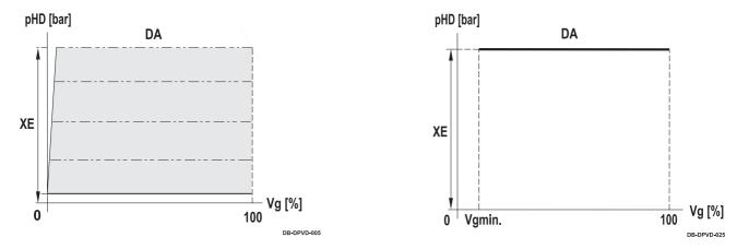
The DA pressure cut-off ensures that the maximum high pressure of the axial piston unit is limited within the regulation range. When a set high pressure value pHD is reached, the axial piston unit swivels in direction  $V_{g\,min}$  and the hydraulic system is protected against damage and overloading.
