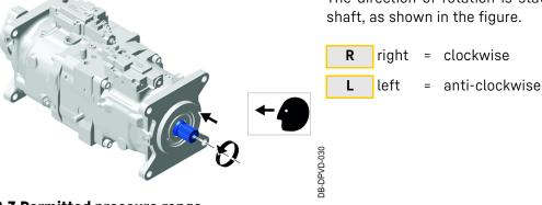
The direction of rotation is stated with view of the driving shaft, as shown in the figure.
