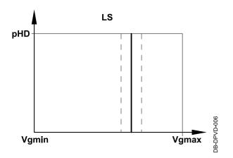
The dynamic characteristics of the control system of variable axial piston pumps can be further improved by load sensing (LS) systems. The LS function is designed as a so-called load pressure reporting system that adapts the volume flow to the current requirements of one or more consumers. It reduces power losses compared to control functions that deliver at maximum volume for a lower volume flow demand.
