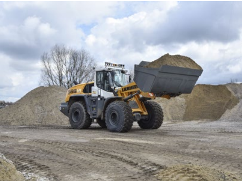
L 566 XPower® transports raw gravel from the flushing fields to the sieving plants
