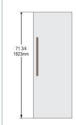
Custom panels should be at least 5/8"(16mm) and a maximum of 3/4"(19mm) thick and they should cover the front of the dedicated cabinet box.
