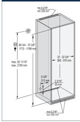
This is a fully integrated refrigerator-freezer appliance designed to be completely enclosed in a dedicated kitchen cabinet. This dedicated cabinet box must be constructed in accordance with the specified dimensions and must allow for sufficient air circulation to ensure proper operation.
