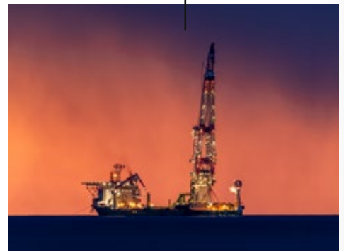
The HLC 295000 Heavy Lift offshore crane with a lift capacity of up to 5,000 tonnes.
