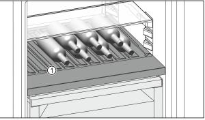
*Fig. 111 Example illustration* (1) Variable bottle rack
